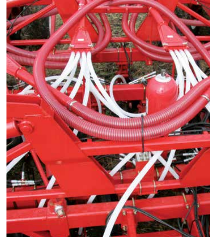
Down force can be adjusted from 200 to 690 lbs depending on spacing and available frame weight
